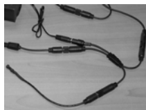
Figure 10 Modular Microphone, properly mated to the Modular AV Harness
