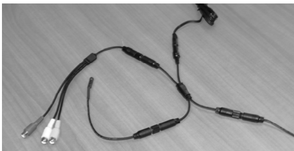
Figure 11 Clockwise, from left: 3xRCA recording cable, connection from the Battery Pack, connection from DT-CAME580 helmet camera and DT-MIC1 Modular Microphone.
