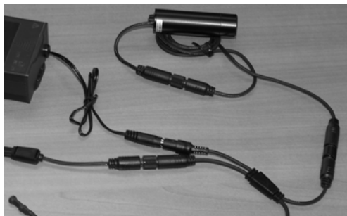
Figure 8 Camera & Video Modular patch cable, properly mated to the Modular AV Harness
